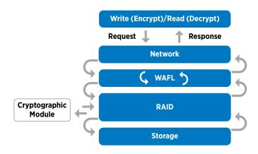
Figure 3) NVE and NAE cryptographic function.
