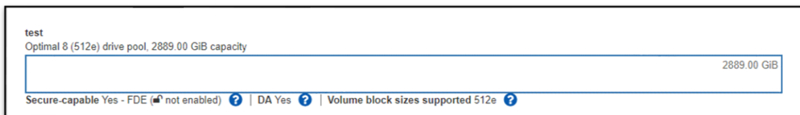
Figure 18) An 8-drive pool created through REST API.
