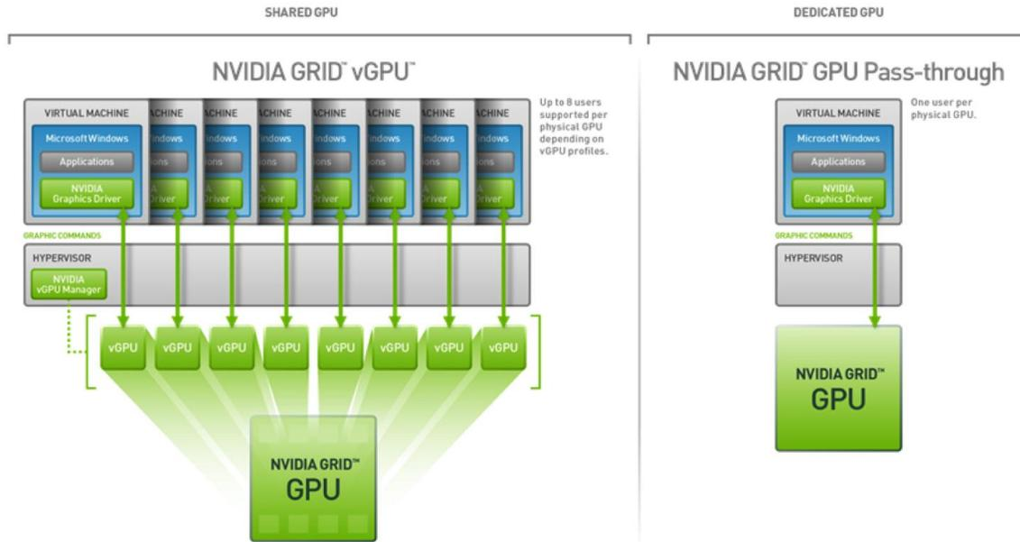
As the first virtualized GPU hardware solution, NVIDIA GRID vGPU allows multiple users to share the graphics processing power of a single GPU. As a result, you can efficiently share GPU resources and broaden the reach of advanced visualization. Each user is assigned a GRID vGPU profile. These profiles correspond closely to the capabilities of typical GPU cards.
