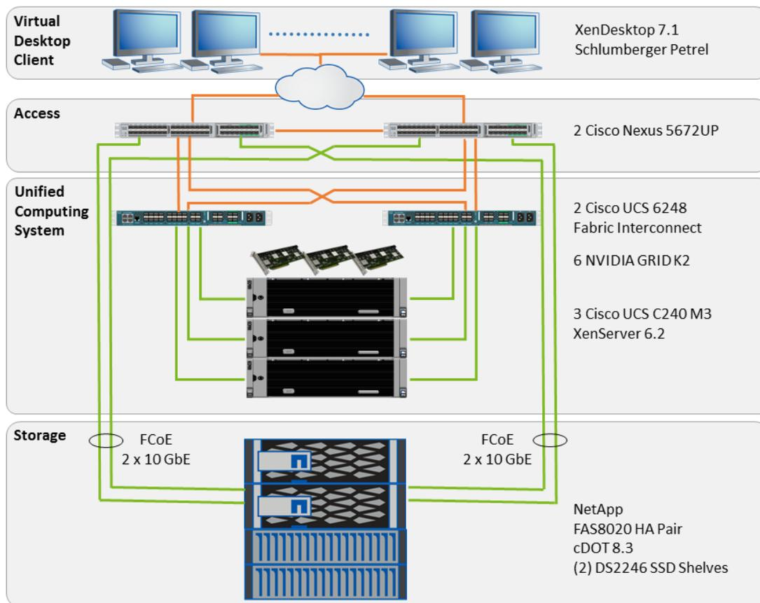
The FAS8020 HA pair served the boot images for the Cisco UCS C240 servers by using the FCoE protocol. FAS8020 storage systems stored the images for each of the VDI clients in volumes located on the SSD drives in the DS2246 shelves. A separate volume on the FAS8020 stored application data. Deduplication was enabled for space-efficient storage of the cloned images. Clustered Data ONTAP 8.3 was selected to run on the storage platform.
