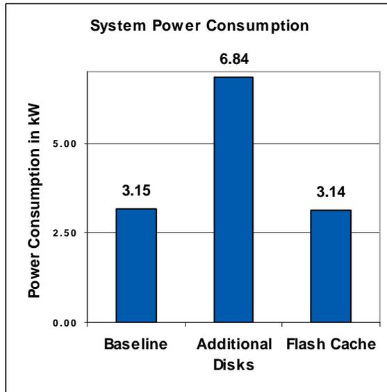
Figure 4) System power consumption
