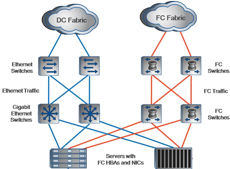
Figure 2) Typical redundant Ethernet and FC SAN infrastructure.
