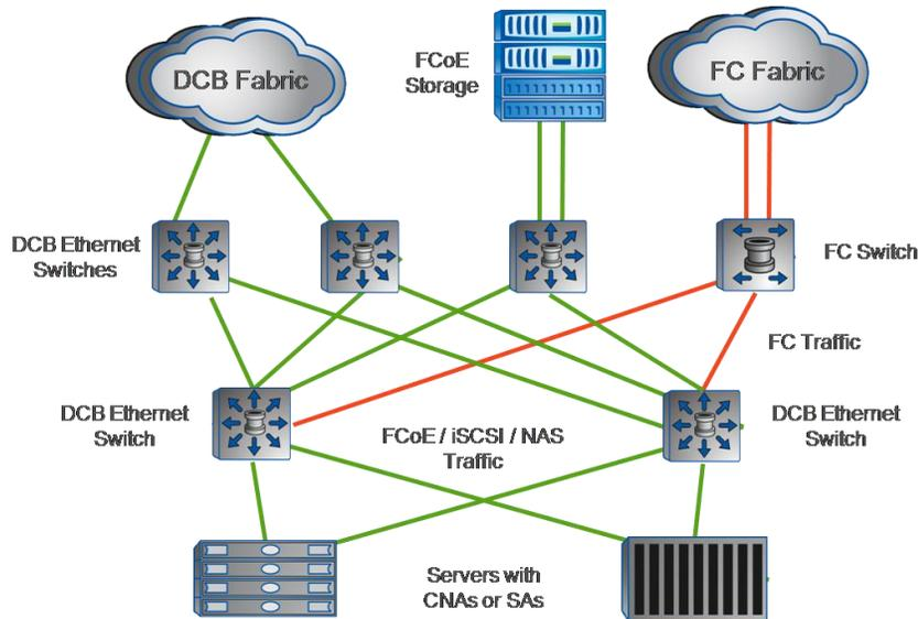
Figure 4) A fully converged network architecture with end-to-end FCoE plus FC investment protection.
