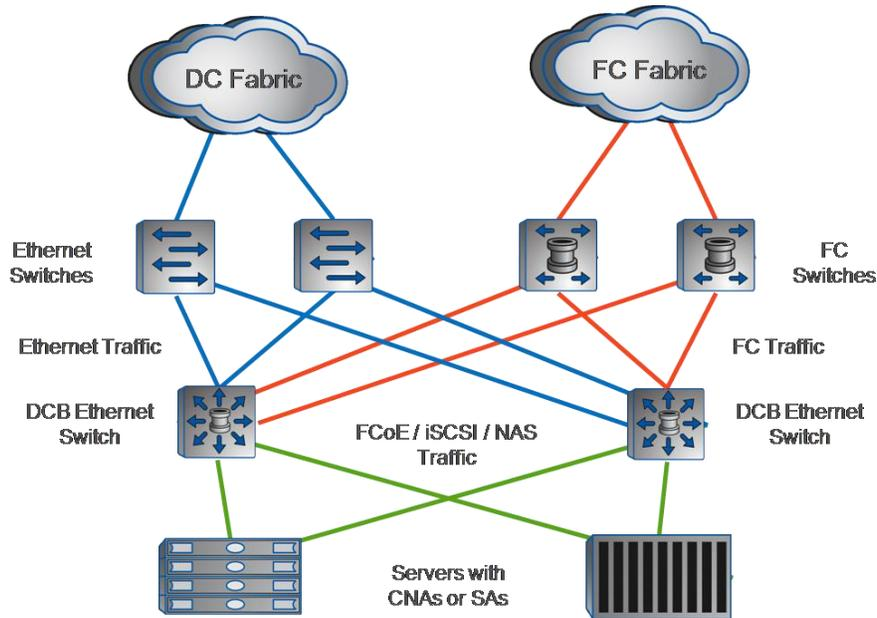
Figure 3) Servers with FCoE adapters attached to DCB edge switches with FCoE enabled simplify the network topology.
