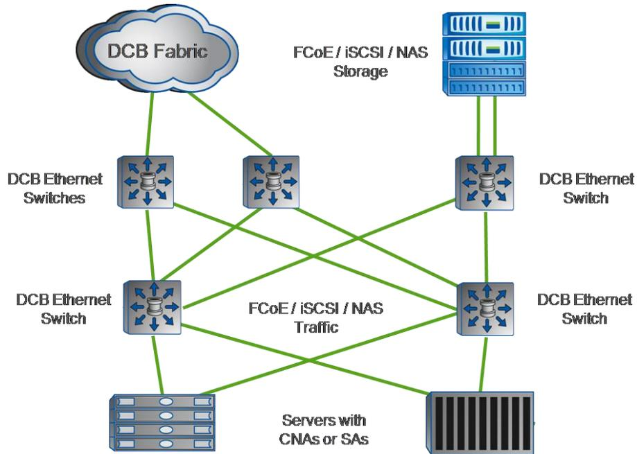
Figure 1) Example of a unified Ethernet fabric using DCB components with FCoE enabled. Switch topology represents a standard edge to core configuration.
