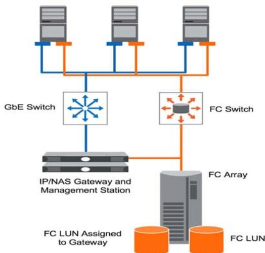
Figure 1) Bolt-together approximation of a unified storage solution.
