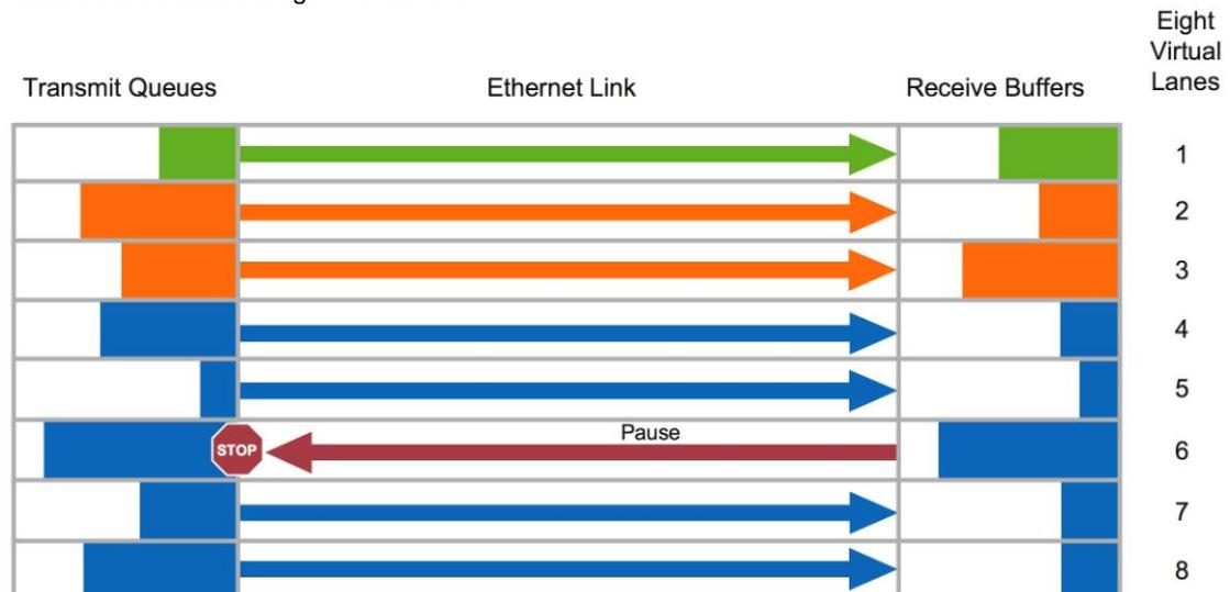
Figure 1) Priority Flow Control allows up to eight prioritized virtual lanes per Ethernet link.
