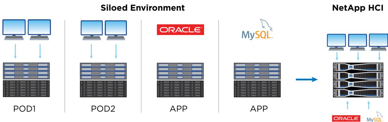
Figure 1) NetApp HCI allows you to consolidate siloed VDI and application environments on a single infrastructure with guaranteed performance and simple management.
