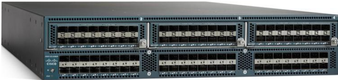
Figure 3) Cisco UCS 6296UP 96-port fabric interconnect.
