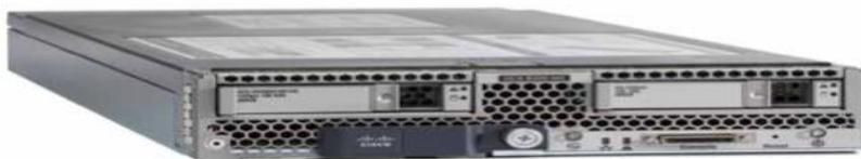
The enterprise-class Cisco UCS B200 M5 blade server extends the capabilities of Cisco UCS portfolio in a half-width blade form factor. The Cisco UCS B200 M5 blade server harnesses the power of the latest Intel Xeon processor scalable family CPUs with up to 3072 GB of RAM (using 128 GB DIMMs), two solid-state drives (SSDs) or HDDs and up to 80 Gbps throughput connectivity.
