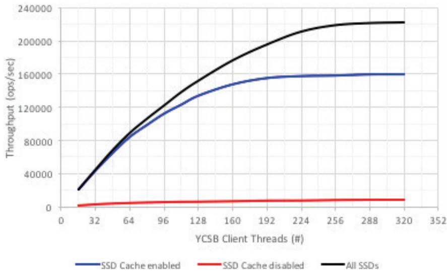
Figure 1) Throughput versus client threads with SSD Cache enabled, SSD Cache disabled, and all SSDs.
