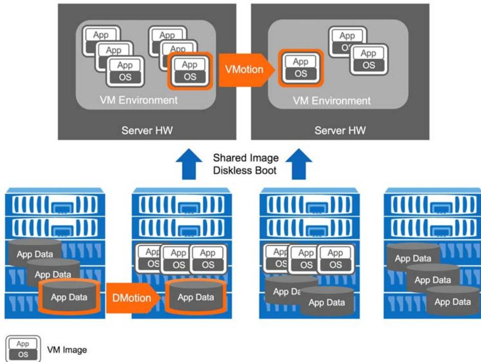
Figure 2) Combining server virtualization with scale-out storage to create a virtual application environment.
