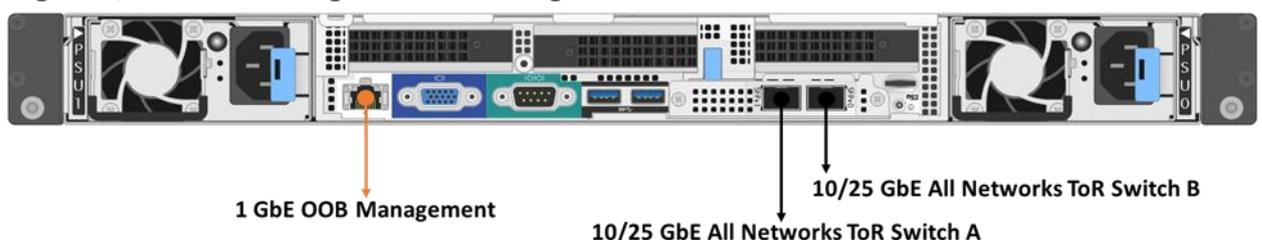
Figure 3) NetApp H410C 2RU 4-node chassis, compute node networking, two cables (option A); all storage, VM, migration, and cluster management traffic is segmented with VLANs.
