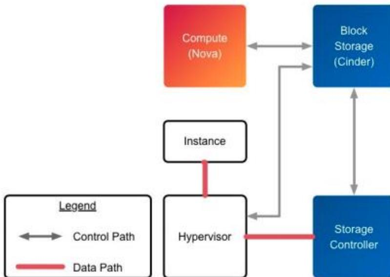
As a management service, Cinder controls the provisioning and lifecycle management of block storage volumes. It does not reside in the I/O (data) path between the hypervisor and the storage controller.
