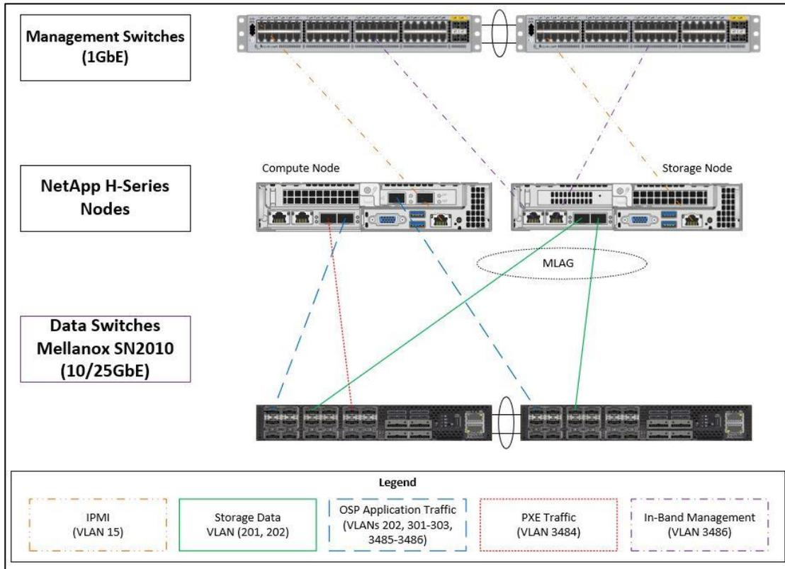
The 1GbE management switches depicted in Figure 5 support both IPMI traffic when booting the OpenStack Platform Director deployed nodes and in-band management connectivity when connected to the NetApp HCI storage nodes. The network ports that each of these are connected to must be configured as access ports tagged to their appropriate VLANs, 15 and 3486 respectively.
