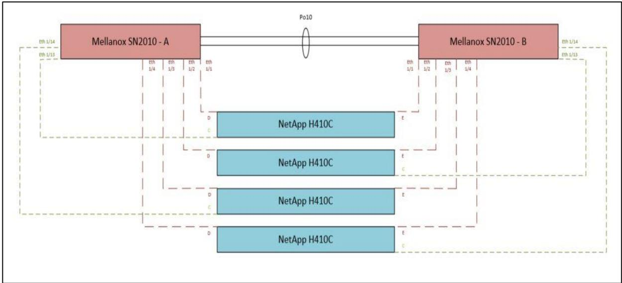
Figure 7) Cabling for four-node storage.
