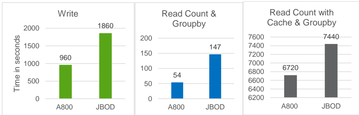
Figure 8) JBOD versus AFF A800 write and read query results on a six-node Spark cluster.
