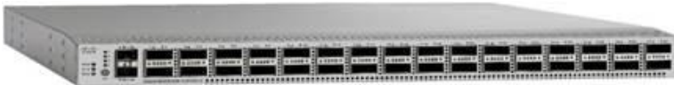
Figure 4) Cisco Nexus switch with NX-OS support for CEE standards and RoCE v1 and v2.
