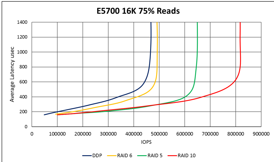
Figure 8) Read-heavy workload expected system performance on E5700.
