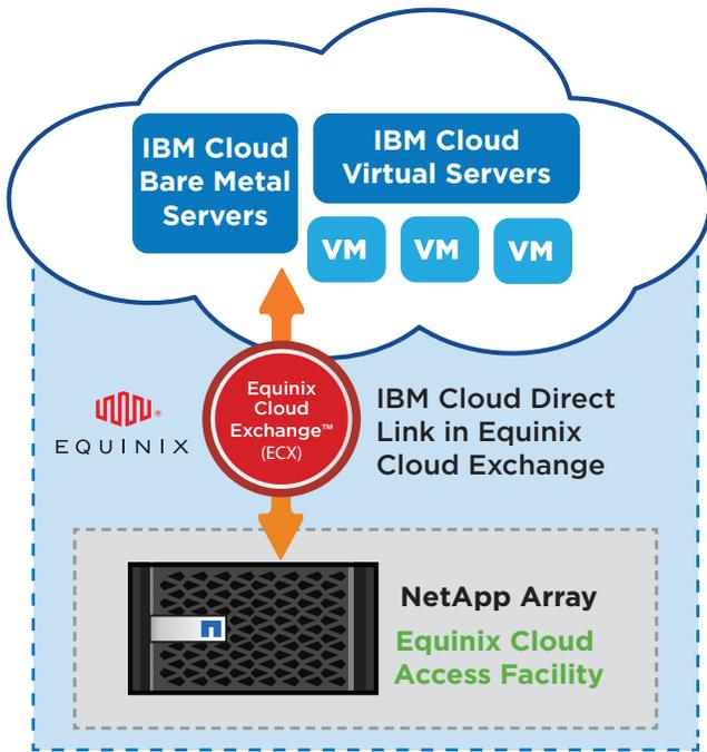
Figure 1: NPS for IBM Cloud: IBM Cloud Direct Link and Equinix Cloud Exchange connect your private storage to IBM Cloud virtual servers and bare-metal servers.
