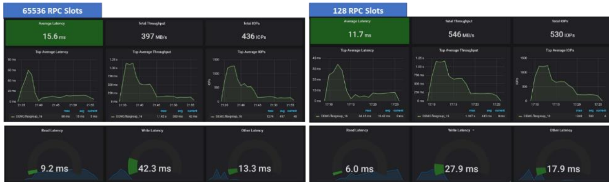
Figure 15) Parallel dd performance: NFSv3 and RPC slot tables; 1MB rsize/wsize.
