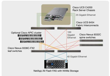
Figure 1) FlexPod integrates Cisco UCS C4200 Blade Server Chassis with Cisco UCS C125 Rack Server Nodes equipped with AMD EPYC processors, with NetApp All Flash FAS Storage, and Cisco Nexus switching.
