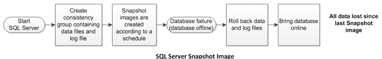
Figure 10) Flowchart of SQL Server database restore with Snapshot image.
