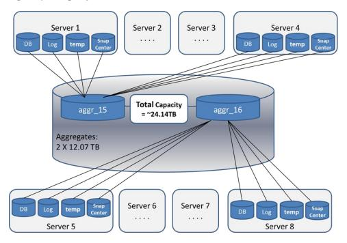
Table 13, located in Appendix A, lists the specifics for each of the AFF8080 storage nodes, including the aggregate, volume, and LUN sizes. Figure 3 shows the storage layout for SQL Server. It shows aggregates aggr\_15 and aggr\_16, one on each storage node, each using 42 x SSDs, leaving one spare SSD per node. With a RAID group size of 21, the configuration yielded 12.07TB of usable storage space per storage node, for a total of 24.14TB of usable space across both nodes.
