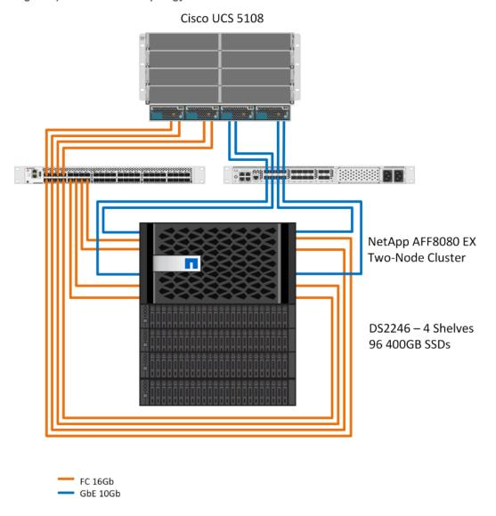
Table 4 and Table 5 show the SQL Server and NetApp hardware and software components used for testing. The storage was configured to make sure of compliance with the AFBP guidelines.
