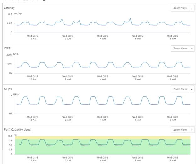
Figure 5) Storage controller IOPS, latency, and performance capacity usage during unplanned storage controller failure testing.
