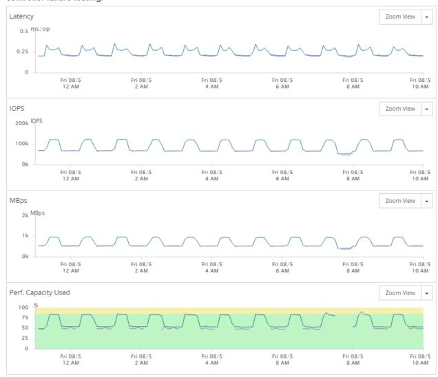
Figure 6) Storage controller IOPS, latency, and performance capacity usage during planned storage controller failure testing.
