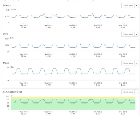
Figure 1) Impact on baseline performance during unplanned storage controller failures.
