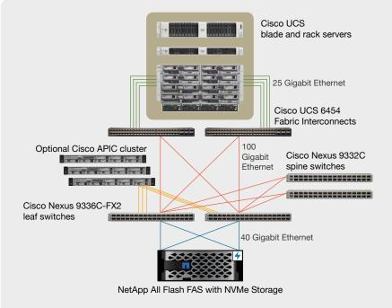
Figure 1) FlexPod is a foundational infrastructure and management solution for your SAP deployments
