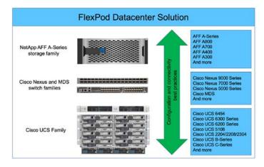
Cisco UCS B-Series and C-Series servers Cisco UCS 6400 series Fabric Interconnects Cisco Nexus 9000 Series switches Cisco MDS Fibre channel switches NetApp All Flash series storage arrays
