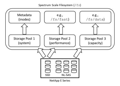
Having three Spectrum Scale storage pools allows the separation of SSDs for data and metadata and the integration of SSD and NL-SAS drives in a single file system. Spectrum Scale always stores the metadata (inodes) of files and directories in the system pool. Equipping the system pool with SSDs improves the user experience for interactive access when users run operating system commands such as 1s -1.
