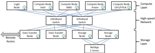
In this example, the dedicated data network is built on InfiniBand, because at this time InfiniBand is the predominant network technology for HPC systems. All nodes are connected through two independent InfiniBand switches to provide high availability. The section called <a href="Spectrum Scale Configuration">Spectrum Scale Configuration</a> describes configurations in which the compute nodes are connected via only one InfiniBand link, to reduce the cost of the overall solution.
