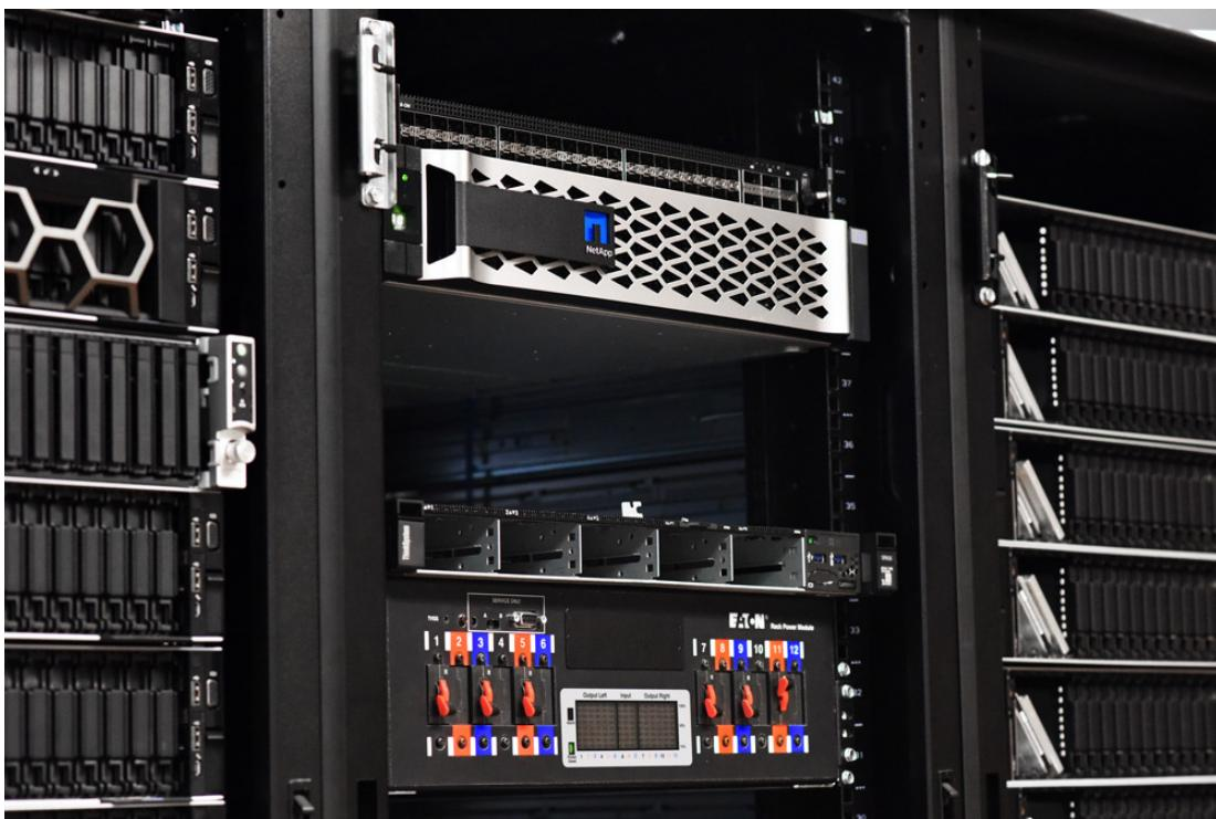
Flipping around to the rear, there are two different designs depending on how the networking is configured; we used the unified, switchless, configuration. The back has a split down the middle for each host with a mirror image on either side. The bottom has the fans and PSUs. At the top of each side are the networking and interconnects, as well as the management ports and USB Ports on the right side.
