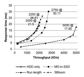
**Figure 1 – Throughput vs. response time for an SPC-1-like workload.** This graph compares the response times as a function of throughput for different hybrid aggregate data placement policies. Table 1 shows the percentage of reads and writes that were serviced by the SSD portion of the aggregate as well as the fraction of the SSD capacity that was used.
