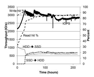
Figure 4 – Extended run of 80/20 filersio with run-length policy. This graph shows a longer term picture of how the run-length policy adapts to the workload.
