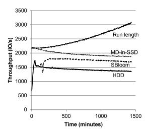
**Figure 3 – Filersio with 80/20 exponential distribution.** This graph shows the throughput achieved by filersio as a function of time for different hybrid aggregate policies when 80% of the I/O is concentrated in 20% of the dataset.
