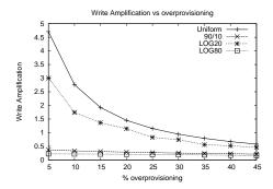
Figure 5: Log: Write amplification vs over-provisioning.
