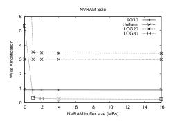
Figure 9: Range container: NVRAM write buffering.
