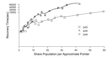
Fig. 12. The effect of the approximate pointers' populations on the time to recover 2,600 secrets using the ring heuristic. In these tests, population, P, was modified by adjusting the size of the region, R, indicated by the approximate pointer; density was kept constant.
