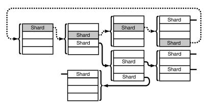
Fig. 9. Recovery example where each approximate pointer indicates a region of four shard names. If shards are produced using a 2 of 4 split, the ring heuristic reveals one recovery candidate based on its circular-linked list structure of *exactly* n, four, shards (shaded shards and dotted approximate pointers). In contrast, the naïve approach of testing paths of length m, 2, would result in many more potential recovery candidates.
