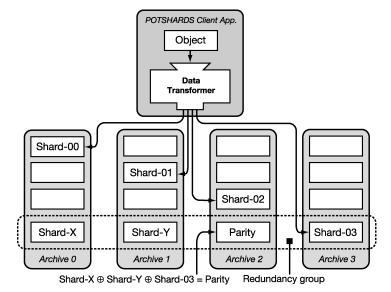
Fig. 1. An overview of POTSHARDS showing the data transformation component of the client application producing shards from objects, and distributing them to independent archives. The archives utilize distributed RAID algorithms to securely recover shards if an archive is lost.
