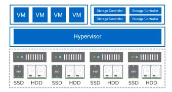
NetApp HCI. NetApp HCI architecture enables independently scale of compute and storage. HCI
