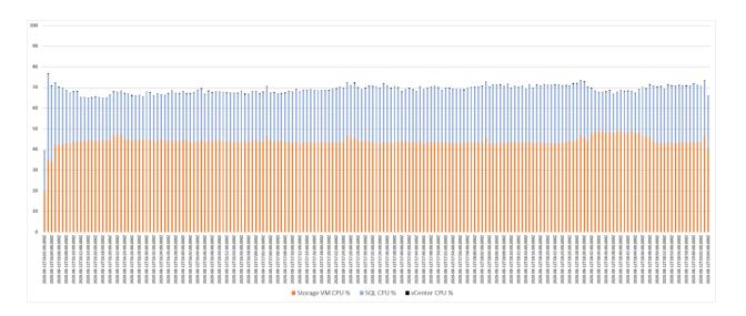
The preceding graph shows the aggregate of all tenants' CPU consumption for a four-node cluster as a percentage of total cluster CPU capacity. When broken out on the individual node level, the CPU consumption picture was almost identical. The storage VM consumed an average of 44% of the node CPU or cluster capacity. The test showed that the CPU overhead for the storage VM was much higher when the cluster was under heavy SQL Server workload.
