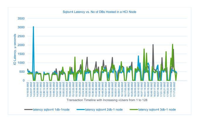
For most of the transaction runs, NetApp HCI I/O latency was under one millisecond with brief spikes up to two milliseconds. The exceptional storage I/O performance of NetApp HCI helped SQL transaction rates remain at a high level as the number of databases scaled up in an HCI node.
