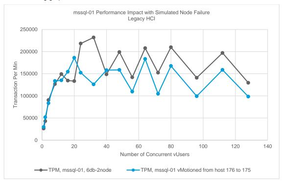
Here you can see that the transaction rate was reduced by as much as 45%. The average transaction performance hit or drop-off at all tested concurrent user levels was about 10% lower.
