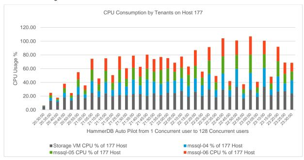
The formula we used to calculate CPU consumption did not figure in hyperthreading, which can normally provide a 15% boost on the CPU capacity in a dual socket system. Therefore, we saw some data points exceeded 100%, which was the net effect of hyperthreading.
