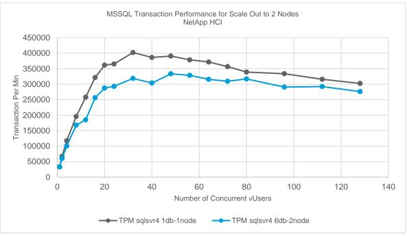
For scale-out performance, the average transaction rate drop-off for conventional HCI was 40.8% while the transaction rate reduction for NetApp HCI was 14.46%. The NetApp HCI relative transaction performance bested conventional HCI by 26.34% (40.8-14.46).
