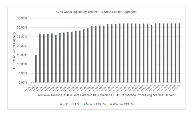
CPU consumption on the NetApp HCI test runs showed that CPU utilization was lower and much more efficient compared similar test runs with conventional HCI.
