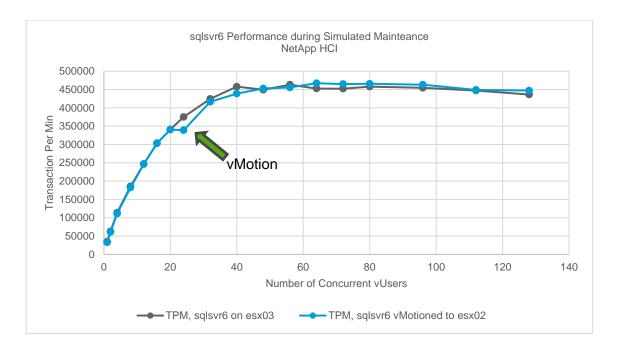
The test results show that there was a minimal effect on SQL Server performance for NetApp HCI during simulated maintenance, which caused a brief 9.6% drop in transaction volume. The performance hit was transient and lasted only about 10-15 minutes before full recovery with the completion of vMotion. Other than that, the transaction performance curves were nearly the same.
