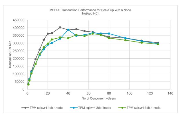
SQL Server OLTP transaction performance is a cumulative effect of the compute and storage of an HCl system. As you scale up the number of databases on an HCl node, some shared resources are in contention such as CPU scheduling, storage IOPS, queue, and so on. Therefore, it is reasonable to expect the transaction rate to come down as the number of hosted databases goes up.
