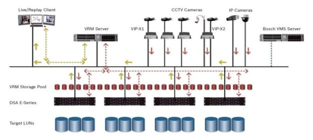
The Bosch VRM solution is designed to meet the needs of the video security market. It is a flexible second-generation IP network video recording technology solution that provides scaling, robustness, and reliability while offering state-of-the-art standard IT components.
