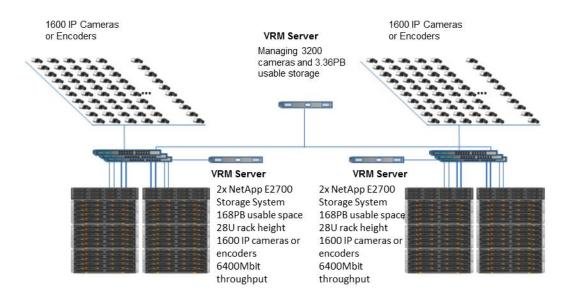
The Bosch VRM solution also works with other video management systems such as Genetec's, giving you the advantage of having a simple and highly scalable recording solution.
