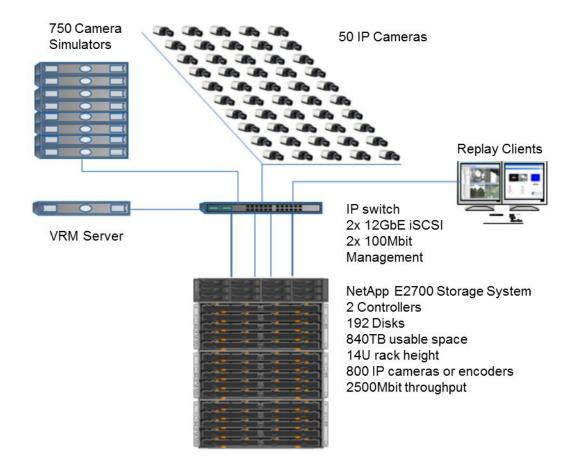
The configuration seen in Figure 9 is a typical setup for a large-scale environment using a video management system such as the Bosch VMS.
