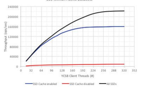
Figure 1) Throughput versus client threads with SSD Cache enabled, SSD Cache disabled, and all SSDs.
