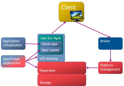
It all starts with the VDI client at the top. That's where the user connects from. To decide which desktop the user is entitled to and how it can connect, a Broker is added. All enterprise solutions have one. This infrastructure component can be as simple as a web interface sending commands to the Platform Management component(s). These Platform Management components are what drive the VDI solution. They manage the creation, resetting, deletion of the desktops.
