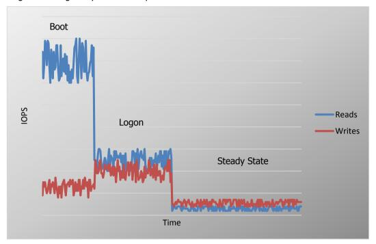
The graph above shows the IO load of a single VDI desktop (as seen on the VDI desktop). On the left there's a high, read IO load (up to several 100s of IOPS) of the boot of the OS. Then the user logs in and a 60% read at about 50 IOPS is seen. Then the user starts working with about 5-10 IOPS at 85% writes for the rest of the day.
