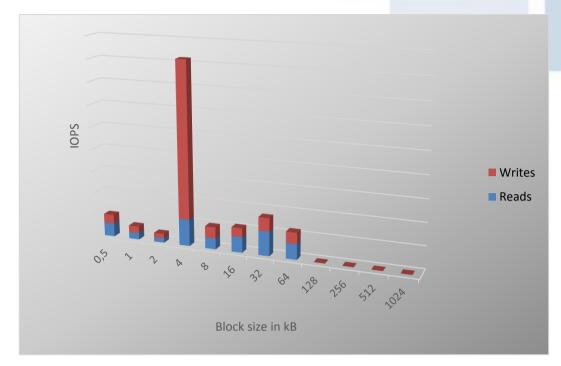
The graph above shows that the typical VDI profile is heavy on writes (85% of all IOPS) and uses mostly 4kB blocks. Other blocks also occur and make it so the average block size is around 10-12kB. Because of this typical VDI profile nature of almost 100% randomness, the storage cache has a hard time making sense of the streams and usually gets completely bypassed leading to less than a few percent of cache hits.
