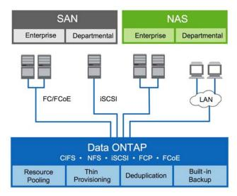
Figure 3) Unified storage foundation—Data ONTAP.
