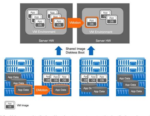
Figure 2) Combining server virtualization with scale-out storage to create a virtual application environment.
