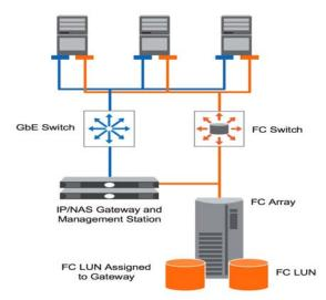
Figure 1) Bolt-together approximation of a unified storage solution.
