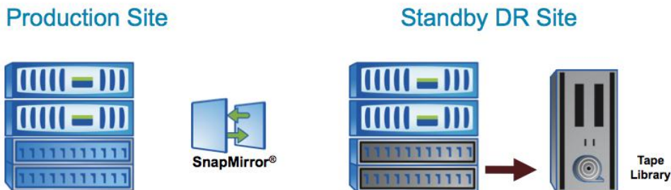
Figure 4) Tape backup operations offloaded to the DR site.
