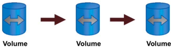
Figure 6) Cascaded volume replication using SnapMirror.
