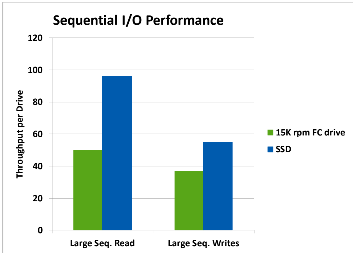
Figure 4) Per-drive sequential I/O performance comparison.
