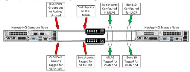
**Note:** Only the two 10/25GbE ports on each storage node must be bonded with MLAG/LACP. The two 1Gb management ports do not need to be bonded.
