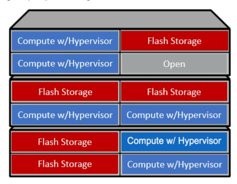
**Note:** The number of storage nodes in a NetApp HCl environment is independent of the number of compute nodes. Usually, deployments have a different number of storage nodes than compute nodes because storage requirements in an environment can vary greatly.
