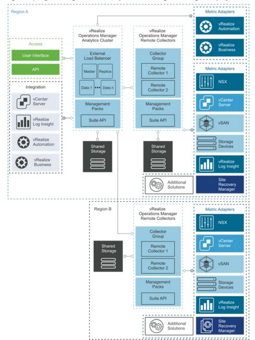
Figure 61) Logical design of vRealize Operations Manager multiregion deployment.
