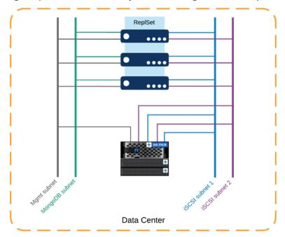
NetApp recommends creating at least one iSCSI LIF for each ONTAP storage node. In this example, there are a total of four iSCSI LIFs. There are two iSCSI LIFS on node1, with each LIF on top of a distinct physical network port on node1. There are another two iSCSI LIFS on node2, with each LIF on top of a distinct physical network port on node2.
