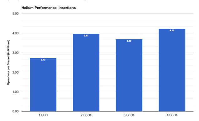
Figure 5) Performance results from increasing the number of SSDs.
