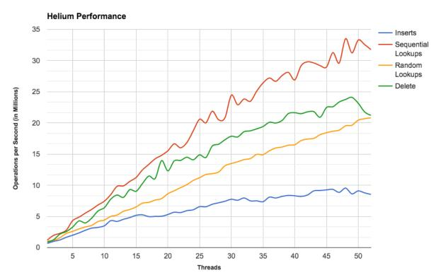
Figure 4) Performance trend from scaling core count, adjusted Helium configuration.
