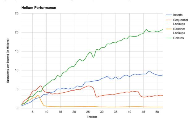
Using basic Helium configurations, throughput for sequential and random lookups reaches a zenith with 8 threads, given that the read\_cache is filled early in the run (8 threads \* (16-byte key size + 100-byte value size + 12-bytes metadata) \* 1 million operations.
