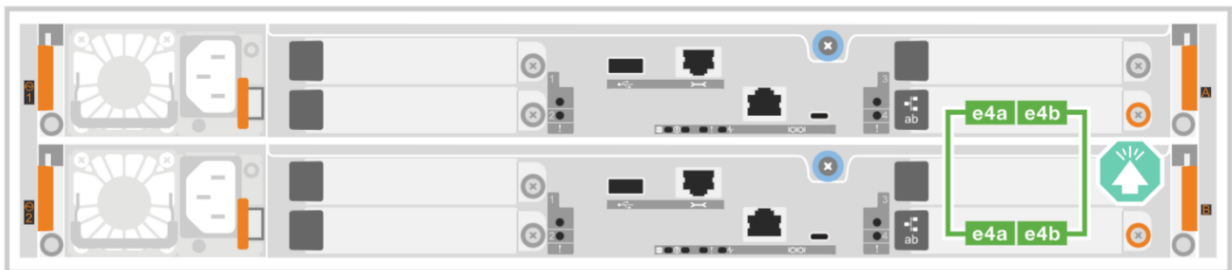
Figure 37) Inter-controller mirroring card port connections.
