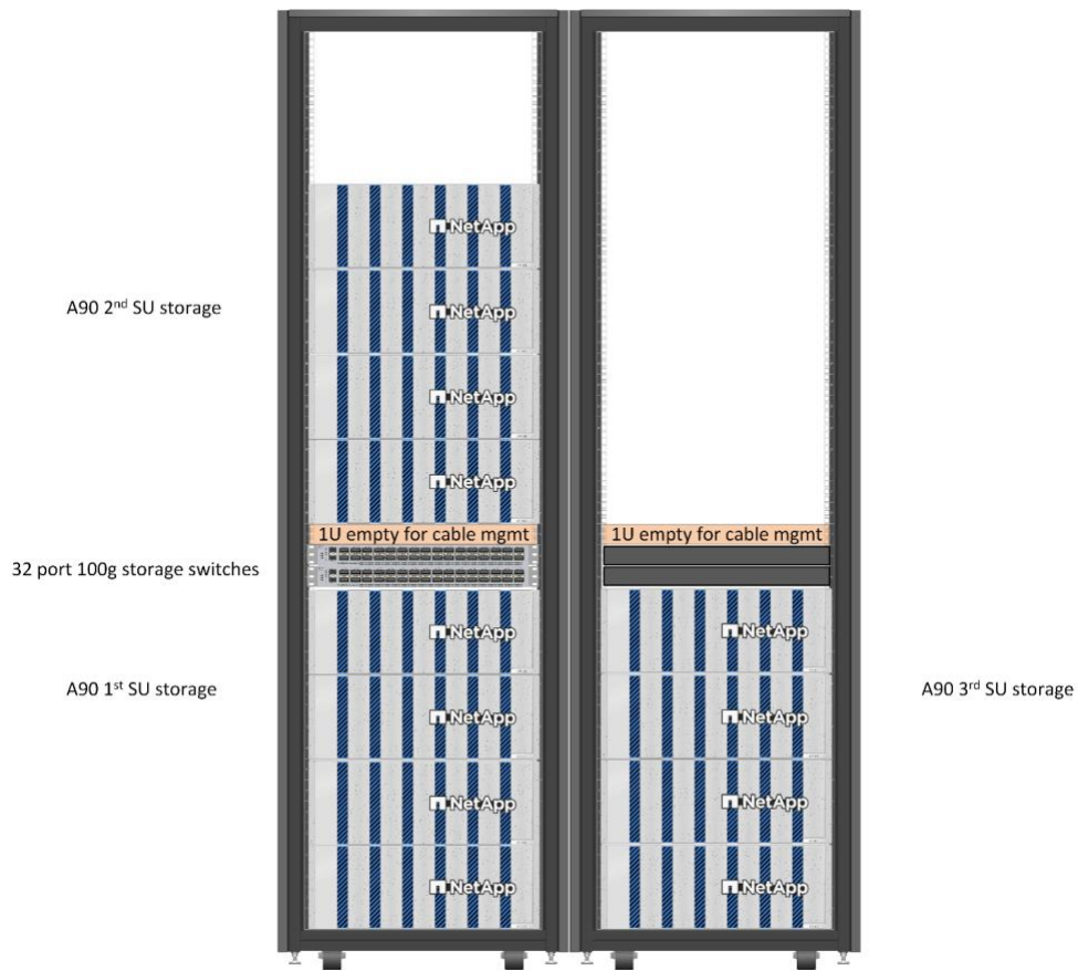
Figure 5) Rack elevations for 3 SU.
