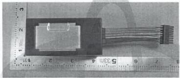
7Vdc 1.45Ah 10.15Wh Rechargeable Li-ion Battery SDI/INR18650-205 可充式鋰離子電池組 型號/Model: NTP2S1P-V 2INR19/65
