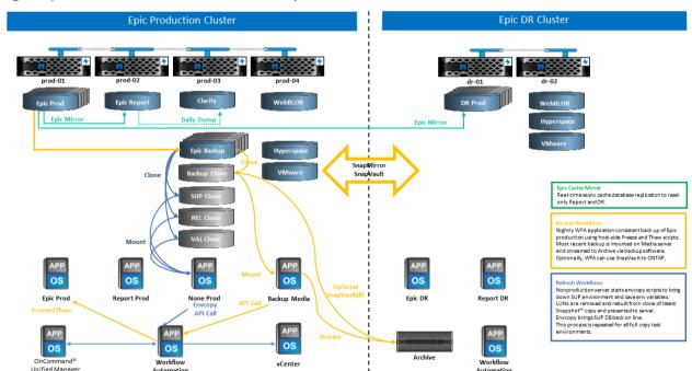
Figure 5) Six-node reference architecture example.
