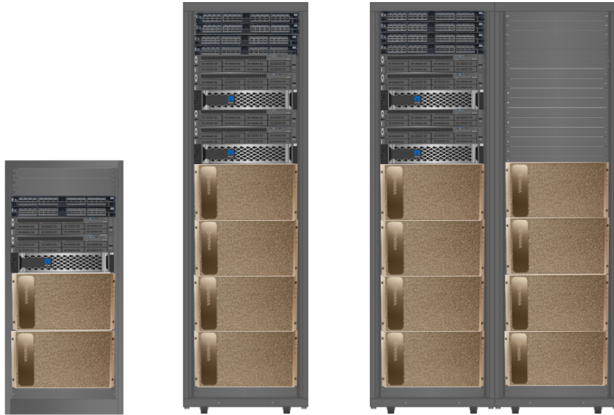
Figure 1) BeeGFS building blocks based on EF-Series with NVIDIA DGX A100 systems
