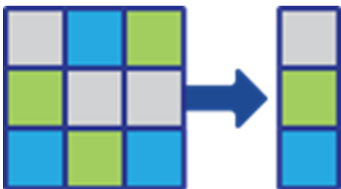
Figure 17) Reducing storage capacity requirements through deduplication.
