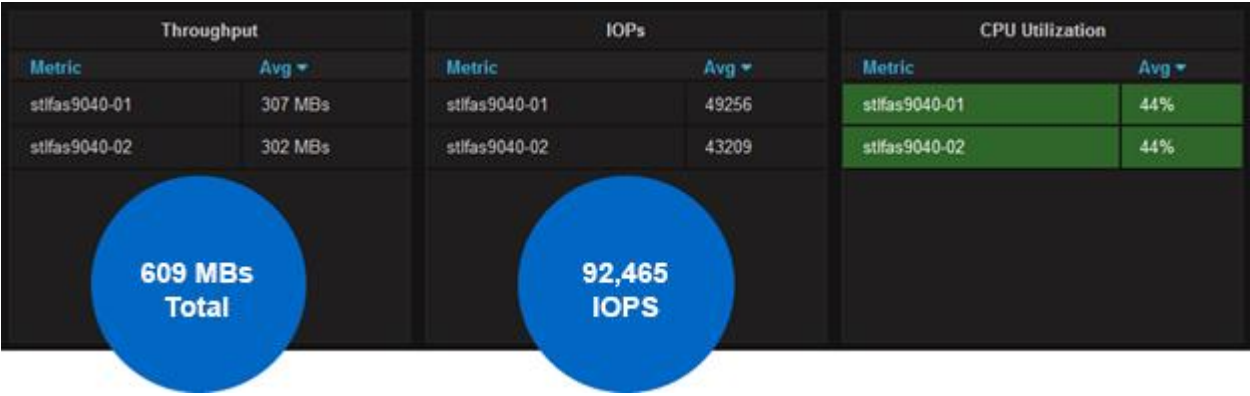
Figure 99) Average CPU utilization, throughput, and IOPS for a FlexGroup volume—AFF A700 HA pair, 128 threads.
