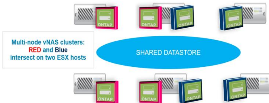
Figure 5) Initial deployment of multinode vNAS clusters.
