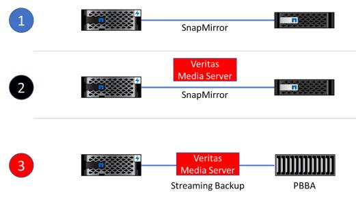
Figure 1. Source and target configurations used in the TCO analysis in Figure 2 below where configuration 1 is a NetApp All Flash FAS (AFF) array to a secondary NetApp FAS array using SnapMirror (blue); 2 is the backup of an AFF array to the same secondary using Veritas NetBackup (black); and 3 is the backup of the AFF array to a leading PBBA using NetBackup (red).
