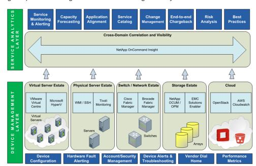
Figure 1) Service management and device management layers.
